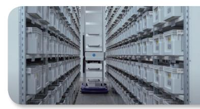
24-hour-operated autonomous guided vehicles were purchased through the Pilot Scheme to save warehouse space and labour costs
